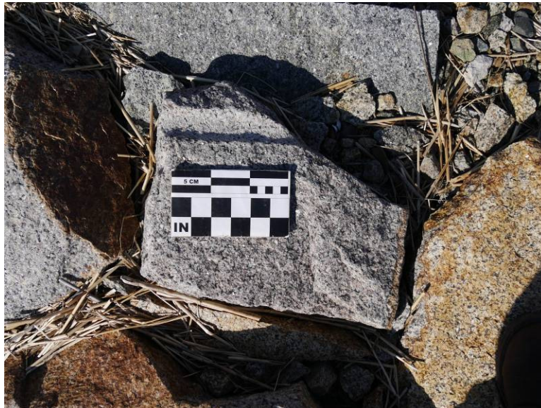
Remains of a round blast blast hole
