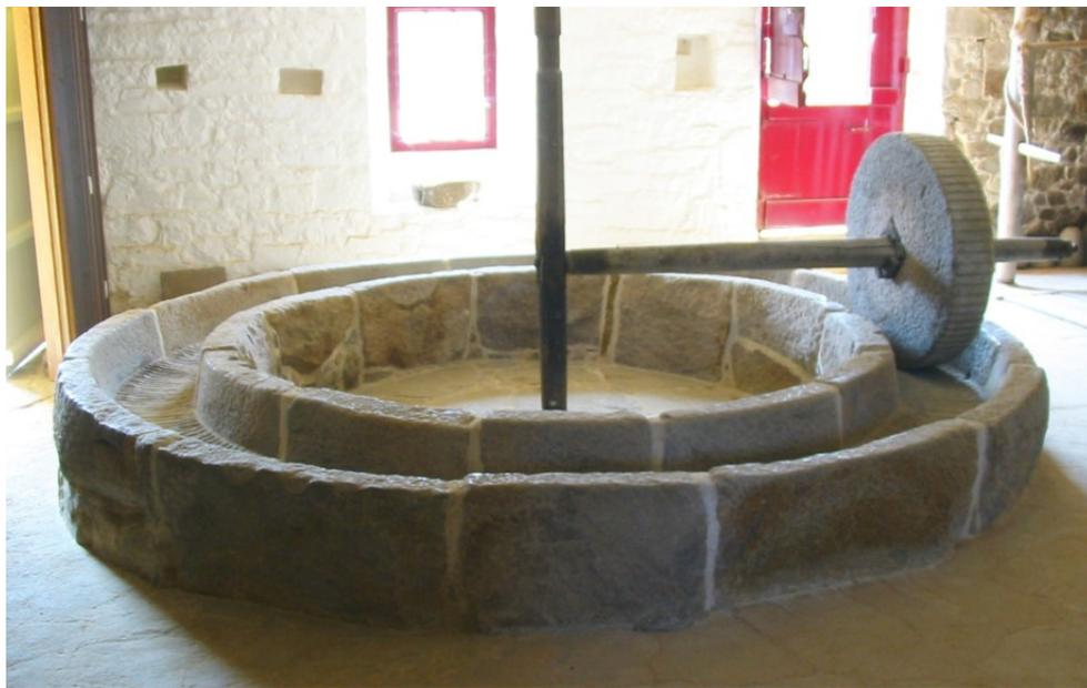
Figure 28 – A multi-segment stone trough held together by mortar from Elms, NJ. This mill was used to crush apples for cider making. (Courtesy of Wikimedia Commons website)
