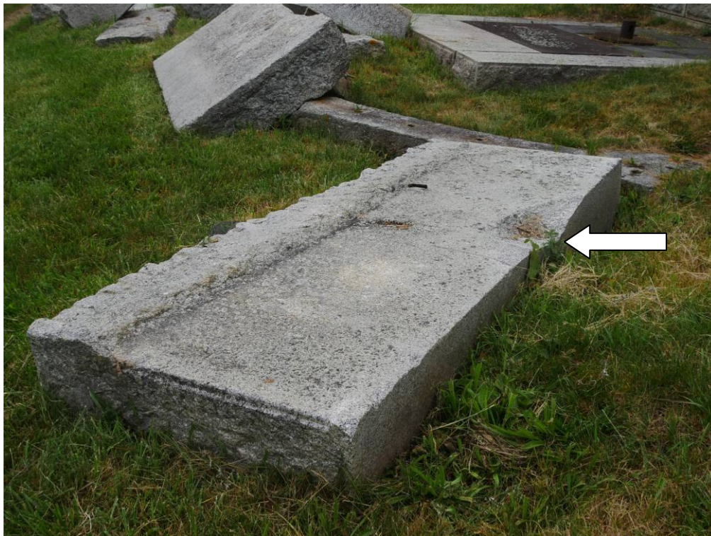
Figure 16 – Block in the process of being finished but abandoned after a large stone flake broke off (arrow)
