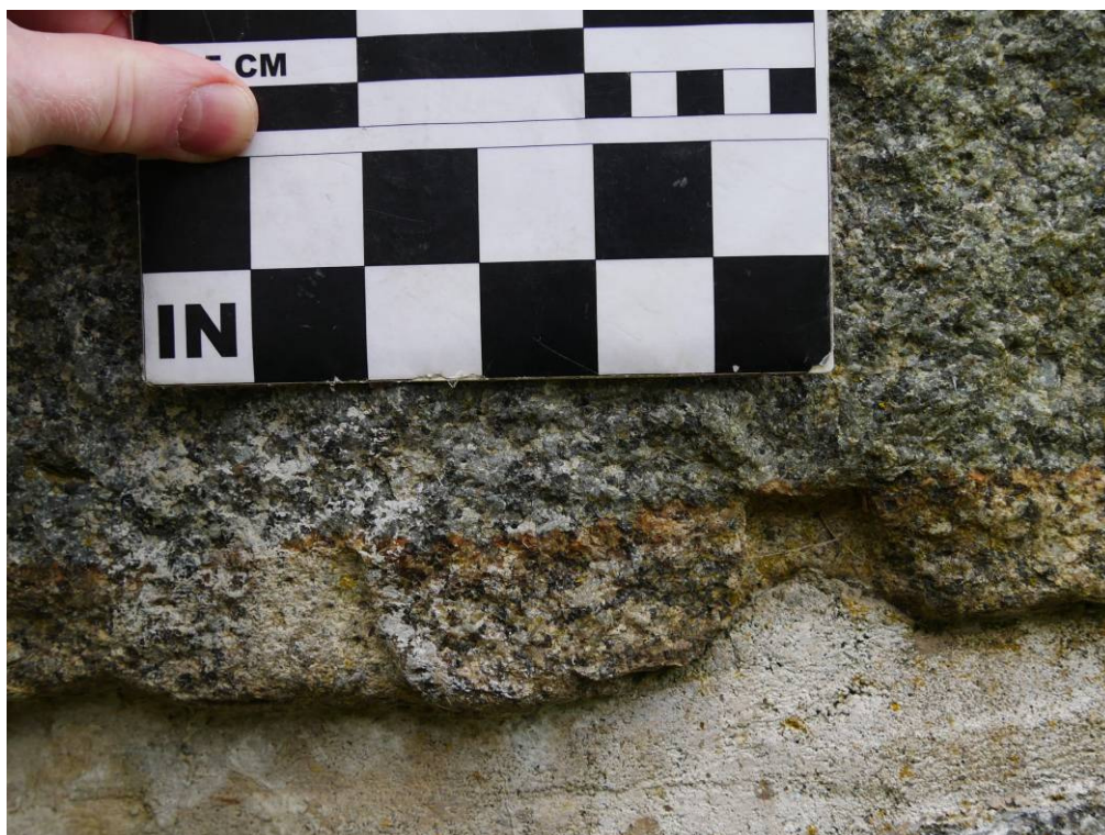
Figure 7 – Hand cut flat wedge holes as seen after the block was split in half. (Holes 1 & 2)
