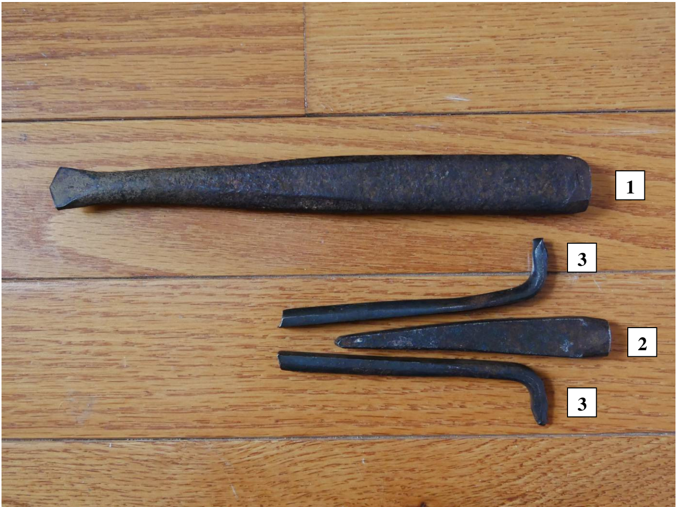
Figure 20 – Tools used for the plug and feather method of splitting stone
