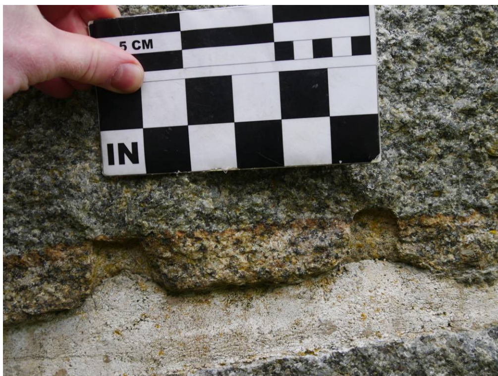
Figure 8 – Hand cut flat wedge holes as seen after the block was split in half. (Holes 2 & 3)
